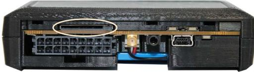
Insert battery into the battery compartment and connect it.
