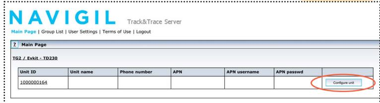
Enter phone number and APN information of the unit. APN information is provided by your GSM operator. If APN user-name and password are not required, leave the fields blank. Click **Send unit configuration** to send the data (SMS).
