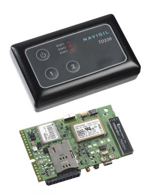
The TD230 is a fully functional tracking application platform with GPS receiver, GSM/GPRS modem, integrated antennas and onboard sensors. Unique features include ultra low power consumption, industry benchmark geofence functionality and SDK for firmware development for customer specific communication protocols, I/O control and application logic implementations.
